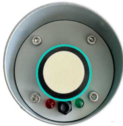
Picture 2: Indicator unit and service probe
